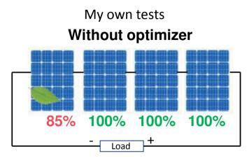
My own tests were done with 4 SA380-72M. The solar power at the time of measurement was about 920 W / m2. The load was 420 Ohm, purely resistive. I shielded some parts of the first panel, or the entire first panel. The voltage from the unshielded panels was from each about 46,5V, regardless of the shading of the first panel. The voltage drop across the first panel was about -1 volts when fully covered. So how can you motivate an optimizer, for me the bypass diodes make about the same effect?
